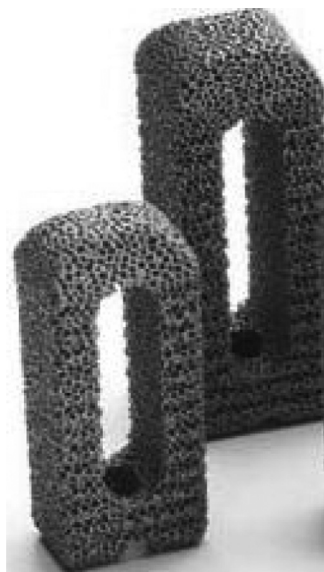
Fig. 1. TM500 (Zimmer Spine, Minneapolis, MN, USA) tantalum intervertebral implant.
